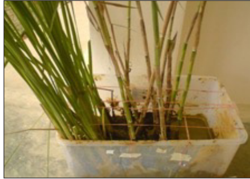
Figure 3. Filtration design model using Cattail Typha Angustifolia
